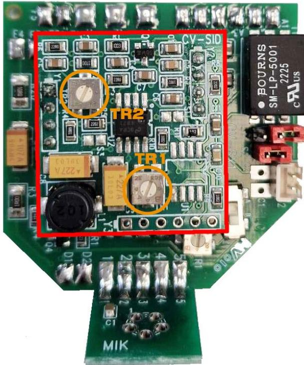
The board in the red box manages the SIDETONE; the main features are listed here below:
